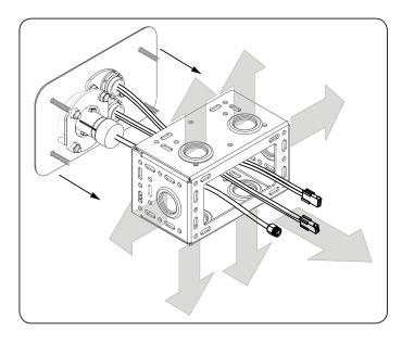
5. Secure the front plate using the fixing screws supplied. Use a TT25 Torx drive bit (supplied) to hand-tighten the screws. Do not overtighten.
