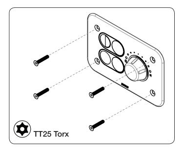
6. Seal edge of front plate with silicone sealant to finish off the installation. (Use anti-pick silicone or silicone sealant of appropriate grade as required.)
