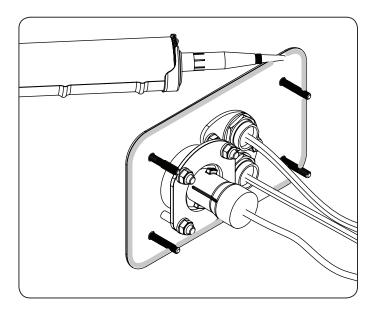
4. Fit control facia plate into position. Feed the cables through any of the half-blind rubber grommets, or through the rear of the bracket box.
