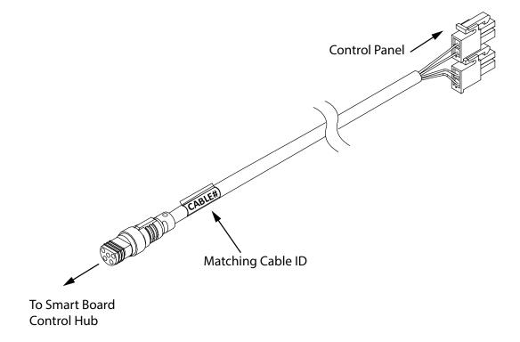
Connect cables to Smart Board eTMV Control Hub.
