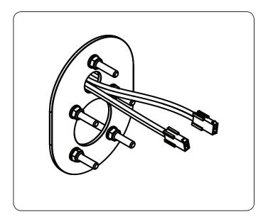
Seal edge of front plate with silicone sealant to finish off the installation. (Use anti-pick silicone or silicone sealant of appropriate grade as required.)
