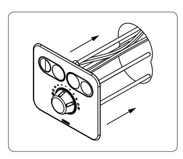
5. Feed cables through. Attach rear plate and secure with nut and washer sets.
