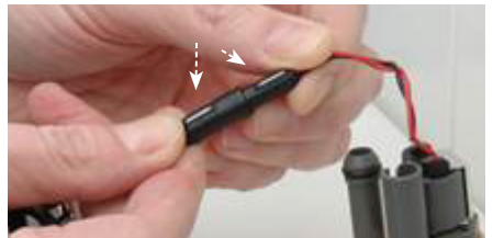
White strips must align on transformer cable IMAGE 18
