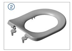
Ensure the plastic sleeves are fitted onto the seat, then fit the assembled hinges onto the seat.
