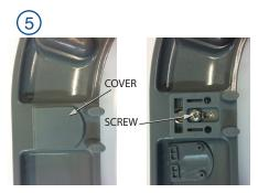
To adjust the position of buffers, pop the cover off the buffer then loosen the screw. Slide the buffer to desired position, then tighten screw to lock the buffer into position.
