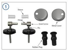
Loosen grub screw and take off hinge from pin. Fit metal cover through the pin, then fit the hinge back onto the pin, then tighten grub screw. Repeat for other hinge. Fit rubber plugs into holes on the pan. Rotate the metal covers out of the way to fit screws through the base of fittings as shown.
