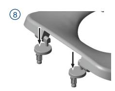
Fit metal covers onto fittings by pushing down.
