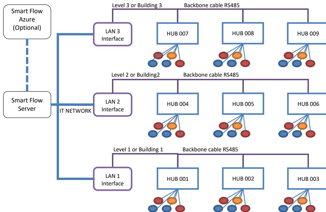
**Note:** The RS485 Backbone Cable and hub to TMV / fixture cabling are not part of the structured cabling network. All cable should be installed by a qualified person.
