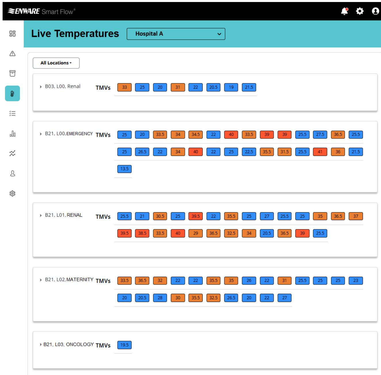
The interface shows live temperature monitoring for Hospital A across five locations. Each location has a list of Temperature Monitoring Points (TMVs) with their current values displayed in colored boxes (blue for 20-25, orange for 30-35, red for 35-40).
