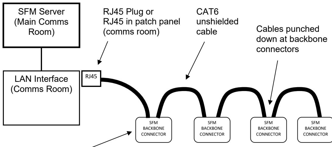
**DESC:** SFM BACKBONE DUAL CONNECTOR SURFACE MOUNT
